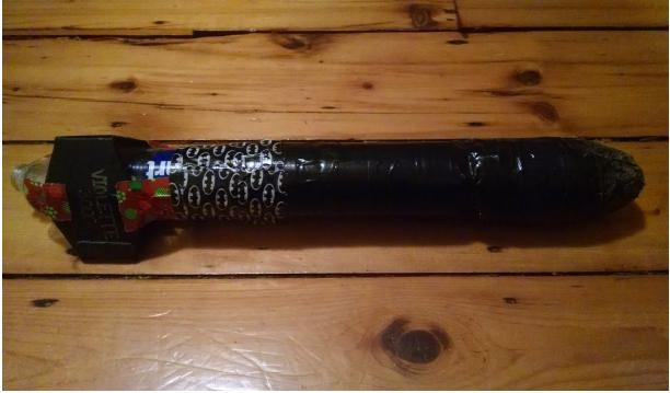
The second final rocket was made of three smart water bottles spliced together with Gorilla Glue Epoxy, again following the method on the US Water Rocket site. The three fins were made from poster board covered in duct tape, and were parallelograms with a width of
